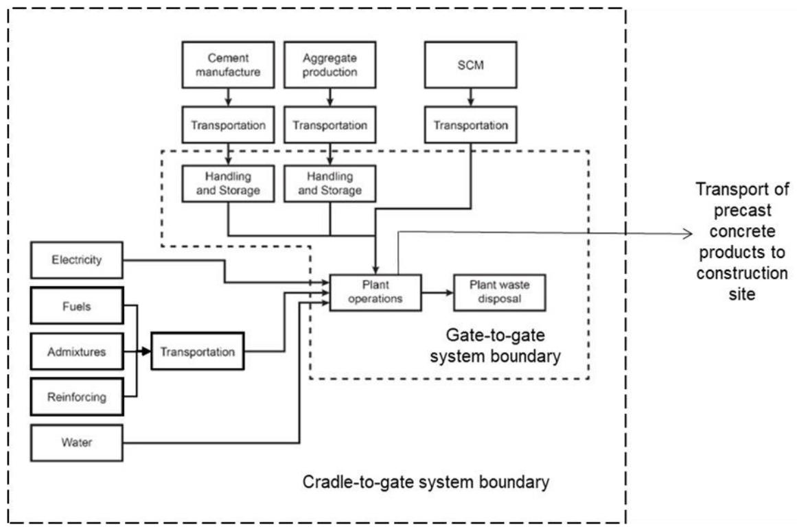
**Figure 2:** System boundary conditions for precast concrete elements, illustrating the difference between unit process (gate to gate) dataset and system process (cradle to gate) dataset (Source: ASTM Product Category Rules for Precast Concrete)
